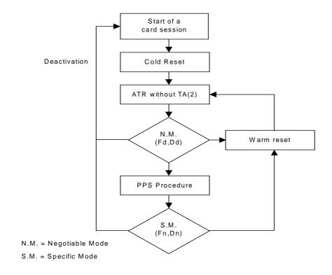
Figure I.1: Modes of operation of a "Type 1 UICC"
