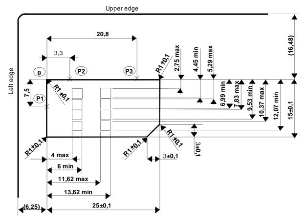
Figure 4.1: Plug-in UICC
