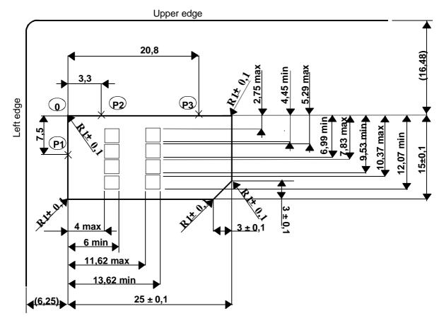
Figure 4.1: Plug-in UICC
