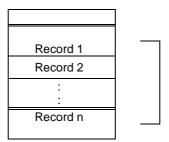
Figure 8.3: Structure of a cyclic file
