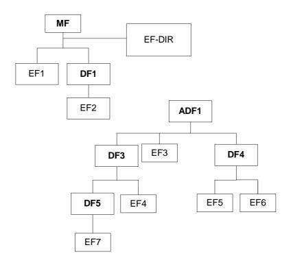
Figure 8.4: Example of a logical structure
