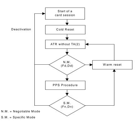
Figure I.1: Modes of operation of a "Type 1 UICC"
