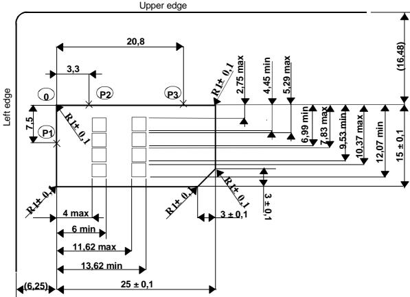
Figure 4.1: Plug-in UICC
