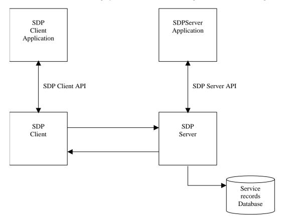
The server maintains a Service Record Database that describe the characteristics of services associated with the server. Each service record contains information about a single service. A client may retrieve information from a service record maintained by the SDP Server by issuing an SDP request.
